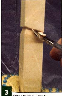
Shape the face. Move to segment 3 and repeat steps 1 and 2. Position the blade on the outside corner of the blank 1/4" down from the stop cut. Cut up to the stop cut to remove about 3/16" from both sides of the face.
