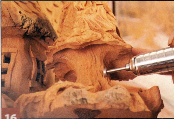
16 Add bark texture to the tree trunk. Use a small thick disc-shaped diamond bit. Make short strokes with just one edge of the disc to create wavy grooves that represent bark texture. Use a tiny knife-edge diamond wheel to add bark texture to the roots.
