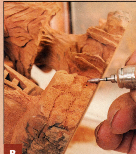
B Carve some bricks. Draw the bricks. Outline them with the small super-coarse flame-shaped ruby bit. Then, soften the edges and make the bricks uneven with the same bit. Buff the bricks with a Scotchbrite disc in a mandrel.
